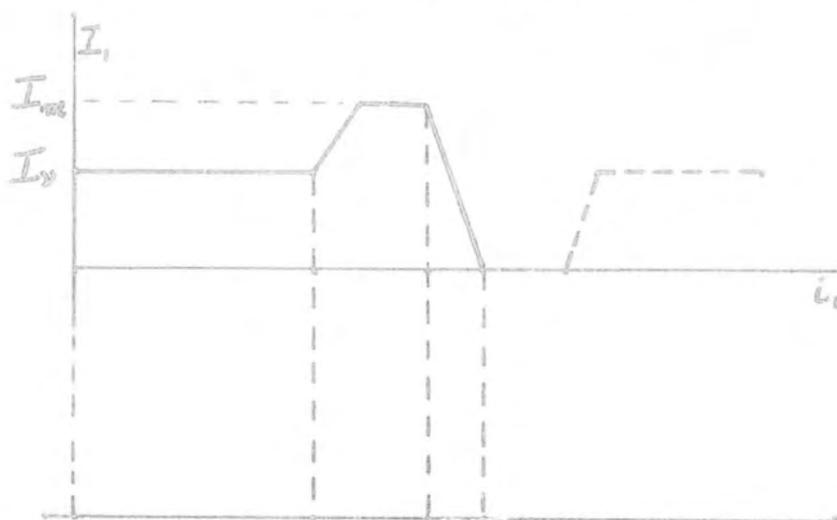
Fig. 3.7 Variation of the output current ( $I$ ) of the control amplifier with spot position ( $i_g$ )
