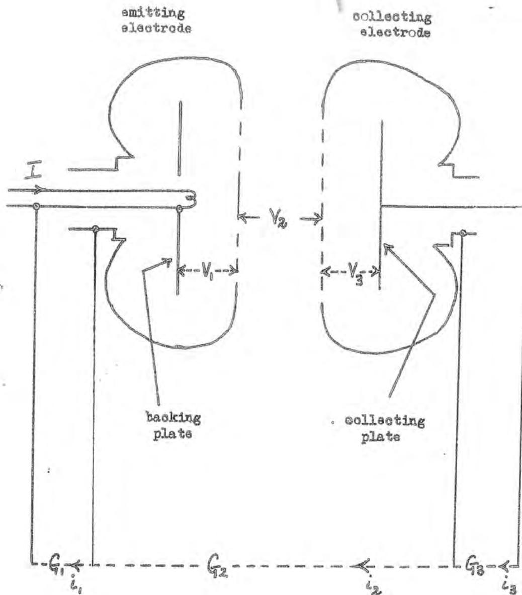
Fig. 2.1: Diagram of the electrodes and current-measuring system.
