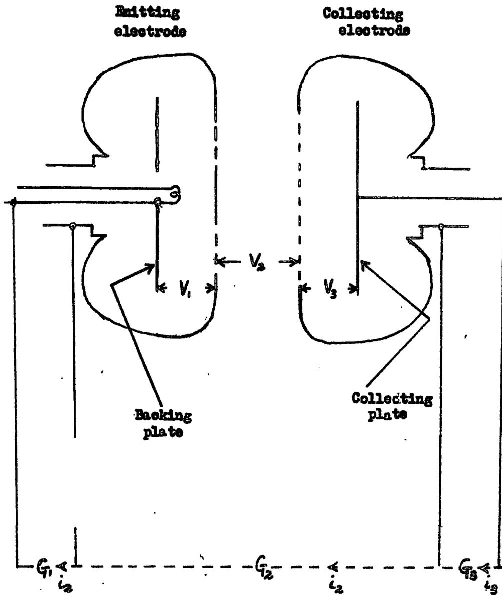
**Fig. 2.1** Diagram of the Electrode and Current measuring system
