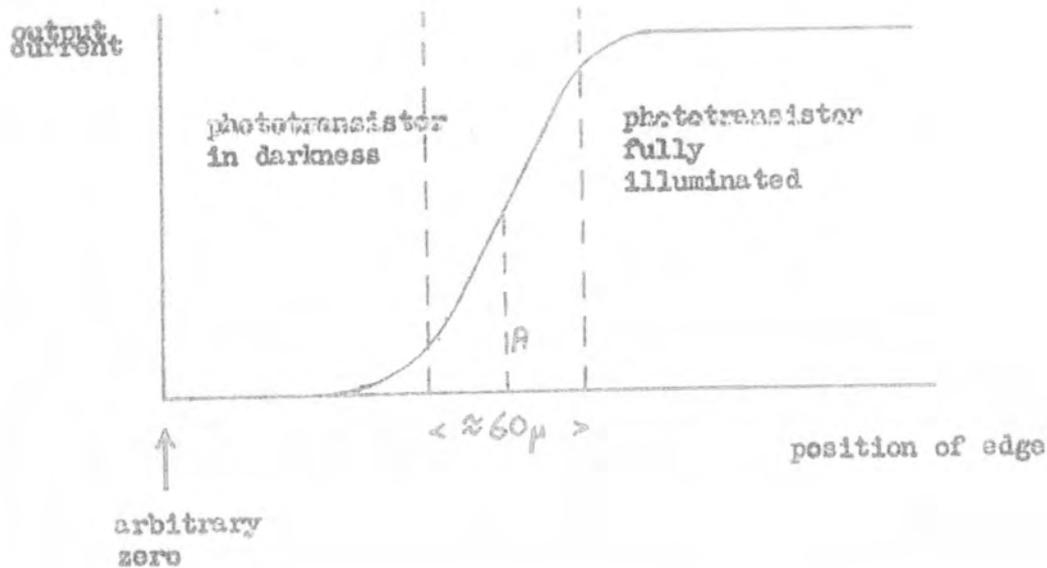
Fig. 3.11 The movement of a straight edge over a phototransistor
