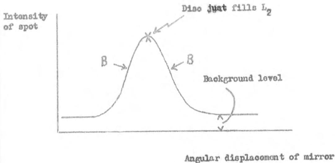
Fig. 3.12 The intensity of the spot impinging of the phototransistors as the disc of light moves across  $L_2$
