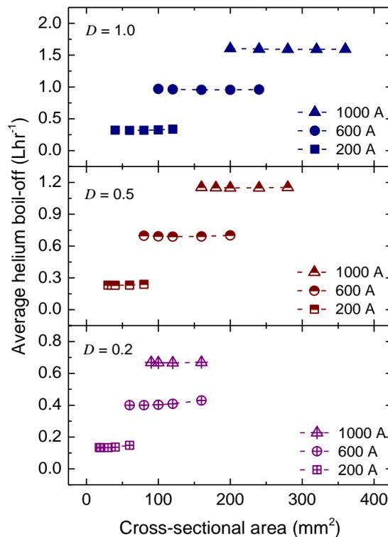
**Figure 5.8** Calculated average helium boil-off (averaged over 10 cycles) for two vapour-cooled brass current leads as a function of the cross-sectional area of each lead carrying a current up to 200, 600 and 1000 A for duty cycles of 0.2, 0.5 and 1.0. The system has no static or sample boil-off and the length of all current leads is 1.0 m.
