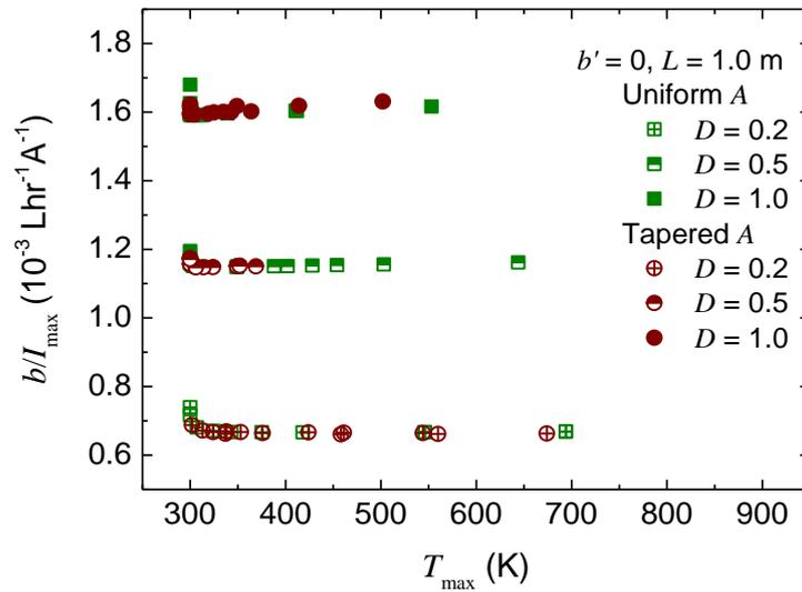
**Figure 5.10** Calculated average helium boil-off per unit current ( $b/I_{\max}$ ) for two vapour-cooled brass current leads as a function of maximum temperature with uniform cross-sectional area and tapered cross-sectional area. The system has no static or sample boiling and the length of all current leads is 1.0 m. The maximum current investigated was 1000 A.
