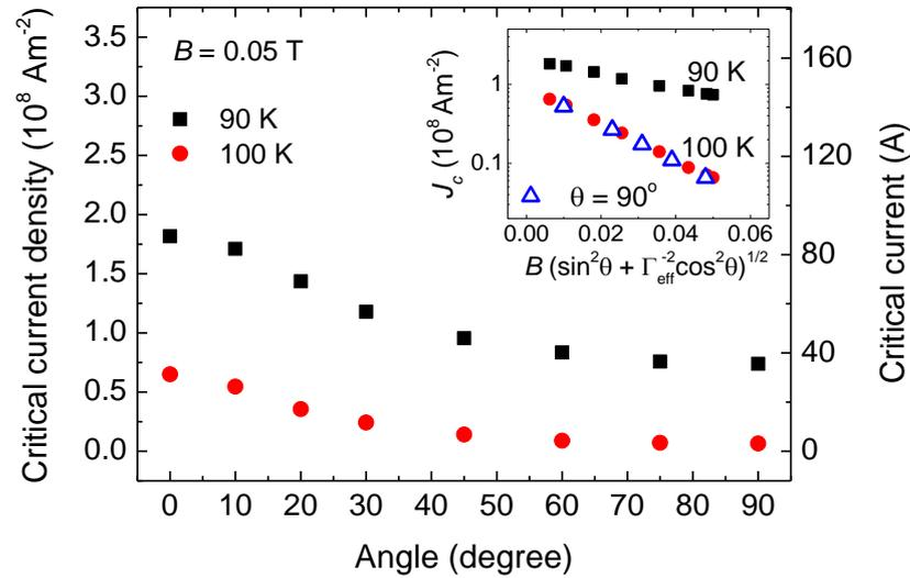
**Figure 7.13** Critical current density of a DI-BiSCCO bare tape as a function of angle between applied magnetic field and the tape surface for the magnetic field of 0.05 T at 90 K and 100 K. The inset shows data replotted as a function of  $B(\sin^2 \theta + \Gamma_{\text{eff}}^{-2} \cos^2 \theta)^{1/2}$ . Data for fields applied normal to the tape surface at 100 K are also plotted for comparison.
