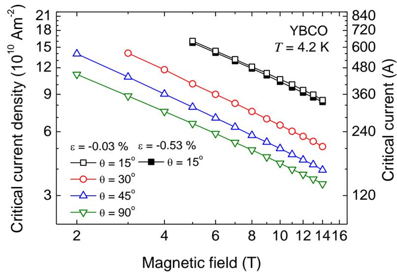
**Figure 5.22** Critical current density of a YBCO tape at 4.2 K as a function of applied magnetic field for different strains and angles between the magnetic field and the tape surface.
