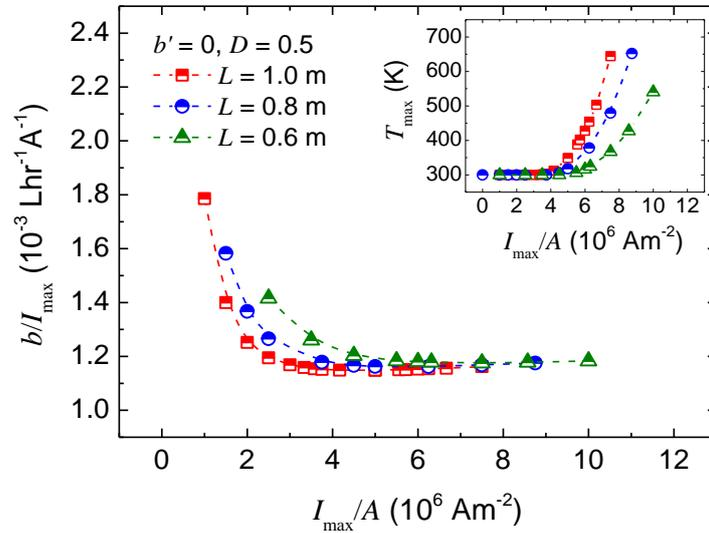
**Figure 5.9** Calculated average helium boil-off per unit current ( $b/I_{\max}$ ) for two vapour-cooled brass current leads and maximum temperature (inset) as a function of the ratio between maximum current and cross-sectional area ( $I_{\max}/A$ ) of each lead without any static or sample boiling for the duty cycle of 0.5 and the current lead's lengths of 0.6, 0.8 and 1.0 m. The maximum current investigated was 1000 A.
