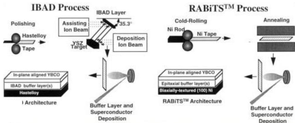
**Figure 3.6** Coated conductor manufacturing process where the textured substrates are prepared by IBAD (left) and RABiTS (right) [137].
