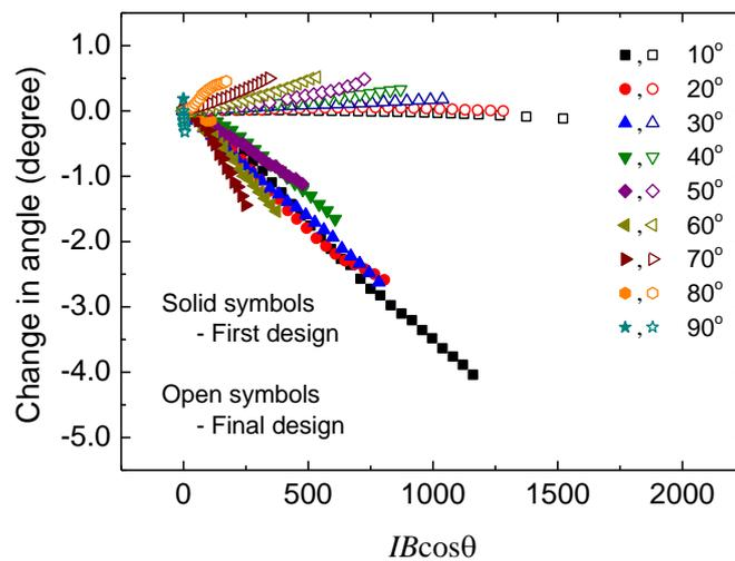
**Figure 5.4** Data from Figure 5.3 replotted as the change in the angle during the  $J_c$  measurement as a function of the product of the current ( $I$ ), the applied magnetic field ( $B$ ) and the cosine of the instantaneous angle between magnetic field and the sample's surface at different starting angles.
