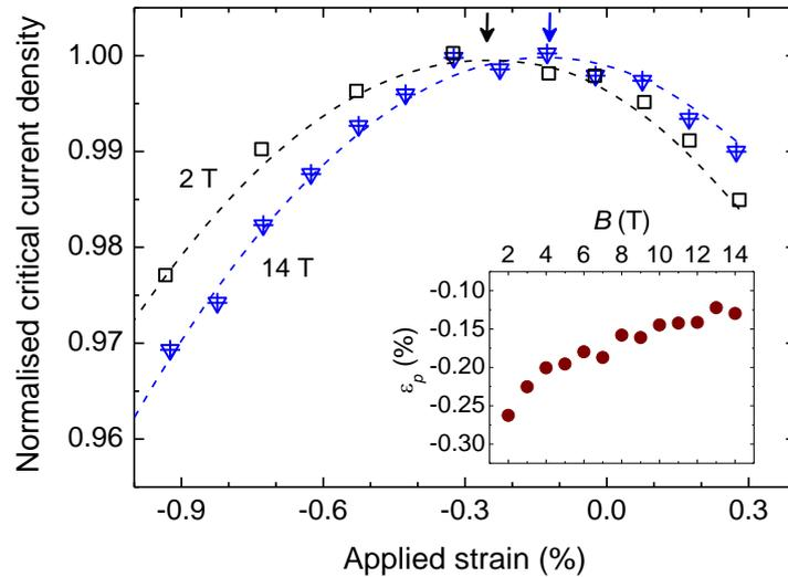
**Figure 6.7** Normalised critical current density of YBCO tape at 4.2 K as a function of applied strain for the magnetic fields of 2 T and 14 T applied normal to the tape surface. Dotted lines are guides to the eye. The arrow shows peak strain ( $\epsilon_p$ ) for each magnetic field. The inset shows  $\epsilon_p$  versus magnetic field.
