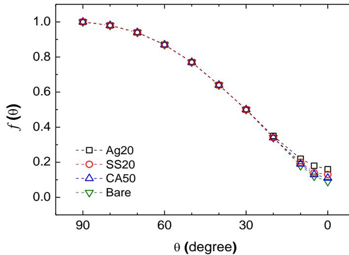
**Figure 4.10** The scaling function  $f(\theta)$  for four different types of the DI-BiSCCO tapes calculated by normalising  $B_{\perp}(\theta)$  with respect to  $B_{\perp}(90^{\circ})$ . The scaling function generally follows  $\sin\theta$  except at the low angles ( $\theta < 20^{\circ}$ ).
