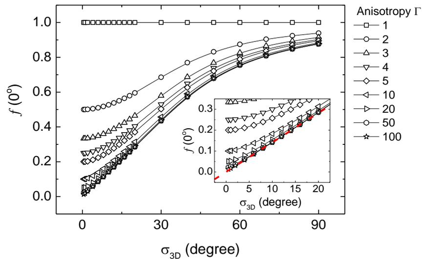
**Figure 7.8** The calculated scaling function at  $\theta = 0^\circ$  as a function of standard deviation of the  $c$ -axis misalignment angle ( $\sigma_{3D}$ ) for various values of the intrinsic anisotropy ( $\Gamma$ ). The inset is the same plot in a different scale. Dotted line in the inset is  $\sigma_{3D} = \sigma_{2D} = 70.9f(0^\circ)$  from (4.3).
