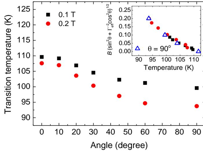
**Figure 7.5** Transition temperature at 1 % of the normal state resistance as a function of angle between magnetic field and the surface of the DI-BiSCCO bare tape for the magnetic fields of 0.1 T and 0.2 T. The inset shows data replotted as a function of  $B(\sin^2 \theta + \Gamma_{\text{eff}}^2 \cos^2 \theta)^{1/2}$  where  $\Gamma_{\text{eff}} = 8.5$ . Data from Figure 7.2 for fields applied normal to the tape surface are also plotted for comparison.
