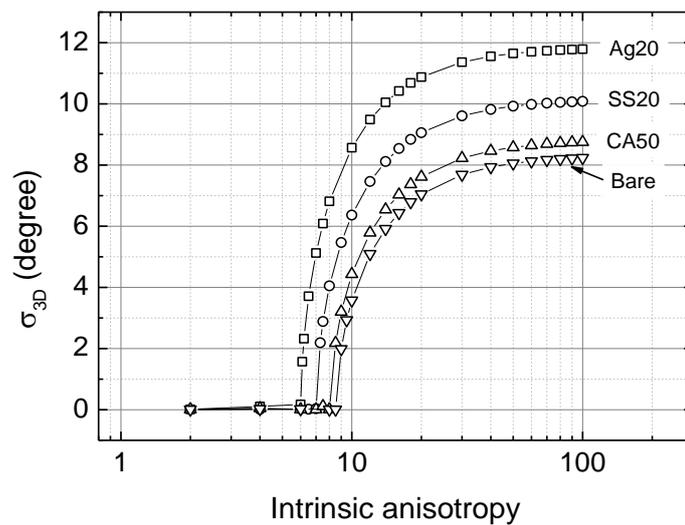
**Figure 7.9** The standard deviation of the misalignment angle ( $\sigma_{3D}$ ) versus intrinsic anisotropy for the DI-BiSCCO Ag20, SS20, CA50 and bare tapes calculated from (7.3) where the scaling function at  $\theta = 0^\circ$  is obtained from the experiments.
