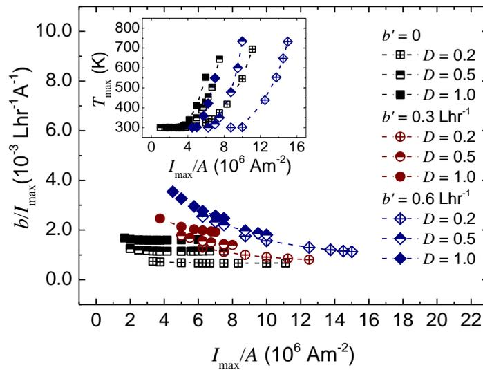
**Figure 5.11** Calculated average helium boil-off per unit current ( $b/I_{\max}$ ) for two vapour-cooled brass current leads and maximum temperature (inset) as a function of the ratio between maximum current and cross-sectional area ( $I_{\max}/A$ ) of each lead with and without static or sample boiling. The length of all current leads is 1.0 m. The maximum current investigated was 1000 A.
