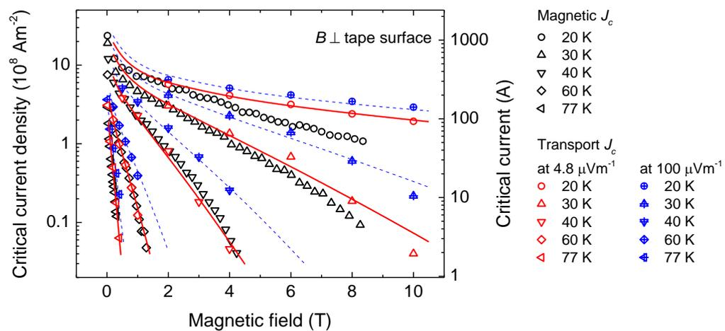
**Figure 7.11** Magnetic and transport critical current densities determined at the electric fields of  $4.8 \mu\text{Vm}^{-1}$  and  $100 \mu\text{Vm}^{-1}$  for the DI-BiSCCO tapes as a function of magnetic field applied normal to the tape surface at different temperatures. Solid lines are fits to the transport data at  $4.8 \mu\text{Vm}^{-1}$  using (6.4) and (6.9). Dotted lines are fits to the data at  $100 \mu\text{Vm}^{-1}$  using the same equations.
