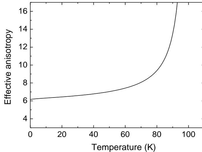
**Figure 7.7** Effective anisotropy of the DI-BiSCCO bare tape as a function of temperature calculated from  $B_{c2}(T,0^\circ)/B_{c2}(T,90^\circ)$  using  $B_{c2}(T)$  from (6.8) where  $T_c(90^\circ) = 101.6$  K,  $B_{c2}(0,90^\circ) = 81.4$  T,  $T_c(0^\circ) = 107.6$  K and  $B_{c2}(0,0^\circ) = 500.6$  T as obtained from the fits in Figure 7.6.
