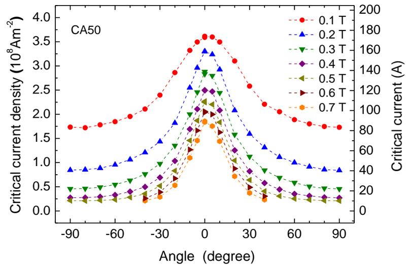
**Figure 4.5** Critical current density as a function of the angle between applied magnetic field and the surface of the DI-BiSCCO CA50 tape at 77 K at different applied magnetic fields.
