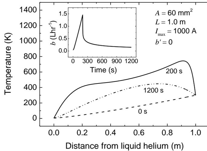
**Figure 5.7** Calculated temperature profile of a vapour-cooled brass current lead with the bottom end immersed in liquid helium while ramping current up to a maximum current of 1000 A in 200 s and then reducing the current to zero without any static or sample boiling ( $b' = 0$ ). The current lead's length is 1.0 m and the cross-sectional area is  $60 \text{ mm}^2$ . The inset shows calculated helium boil-off as a function of time.
