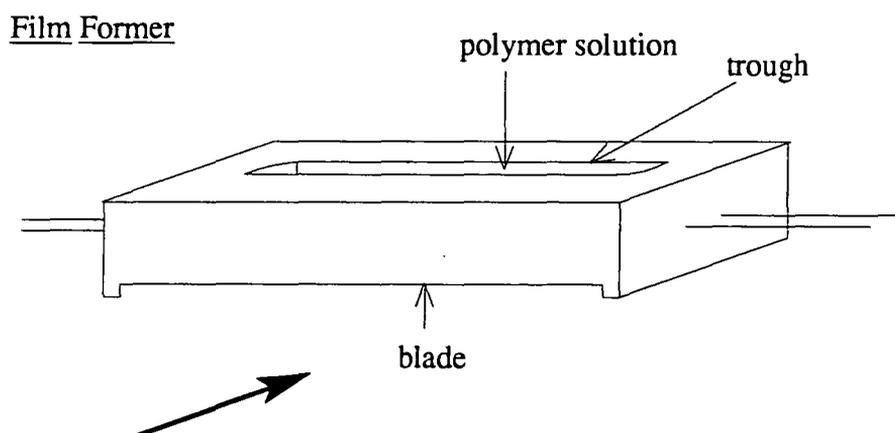
The film former is placed on a clean film of Mylar (about 20 x 30cm). The trough is filled to about 2mm depth with polymer solution, and the former drawn across the Mylar in the direction of the arrow.
