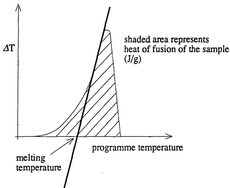
The melting temperature is found by drawing a line through the steepest point on the forward edge of the melting peak and extrapolating it to the temperature axis (Fig 4.10). The percentage crystallinity is calculated as the ratio of the heat of fusion (J/g) of the sample to that of a 100% crystalline material. An indication of the purity of the sample can be obtained from the melting range.
