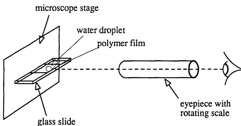
An eyepiece with rotating scale enables measurement of the relative height,  $h$  and base width,  $\omega$  of the drop (Fig 4.7).
