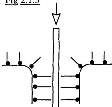
Langmuir-Blodgett deposition on a hydrophobic polymer substrate
