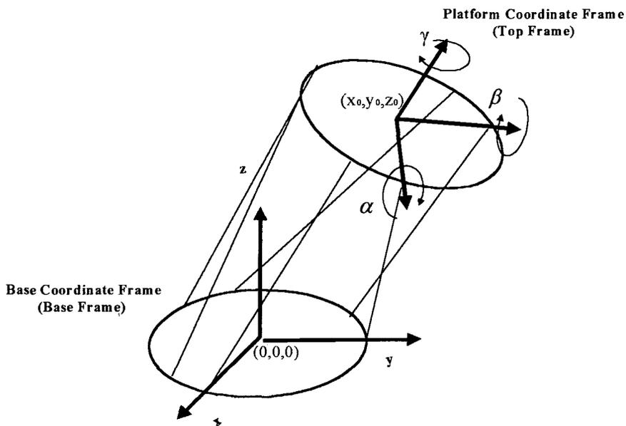
**Figure 5-1** Basic Geometrical model of Stewart platform
