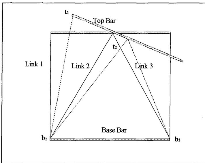
**Figure 3-3** Parallel linkage mechanism for two-dimension, 3D, case
