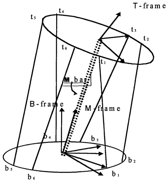
**Figure 5-2** Equivalent geometrical model of Stewart platform
