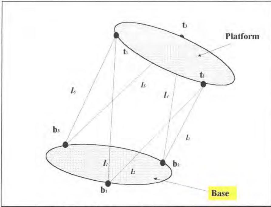
Figure 3-8 Alternative six-link structure.
