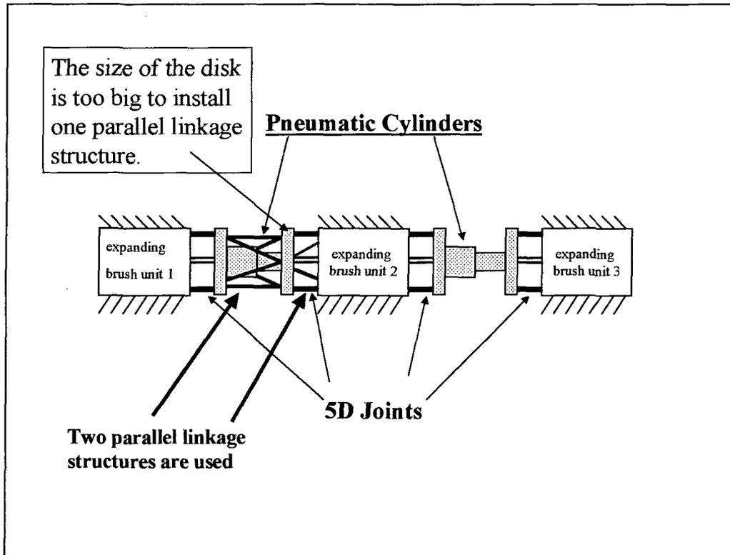
**Figure 3-7** Two parallel linkage mechanisms are used
