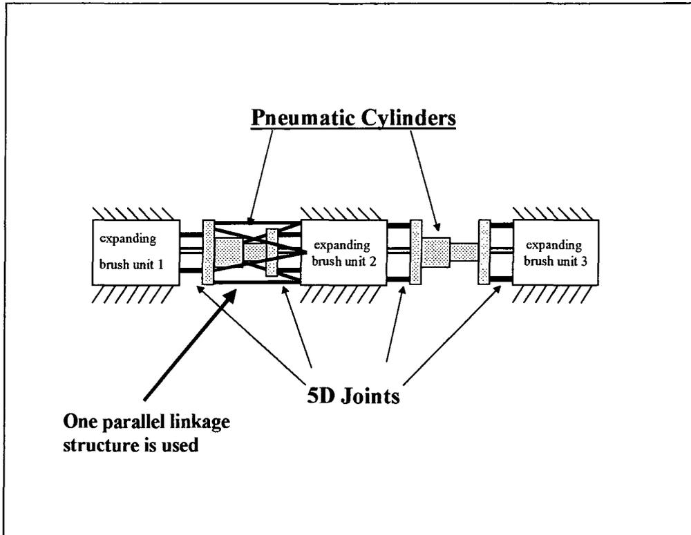
**Figure 3-6** One parallel linkage mechanism is used
