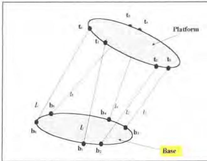
**Figure 3-4** Parallel linkage mechanism for three-dimension, 6D, case
