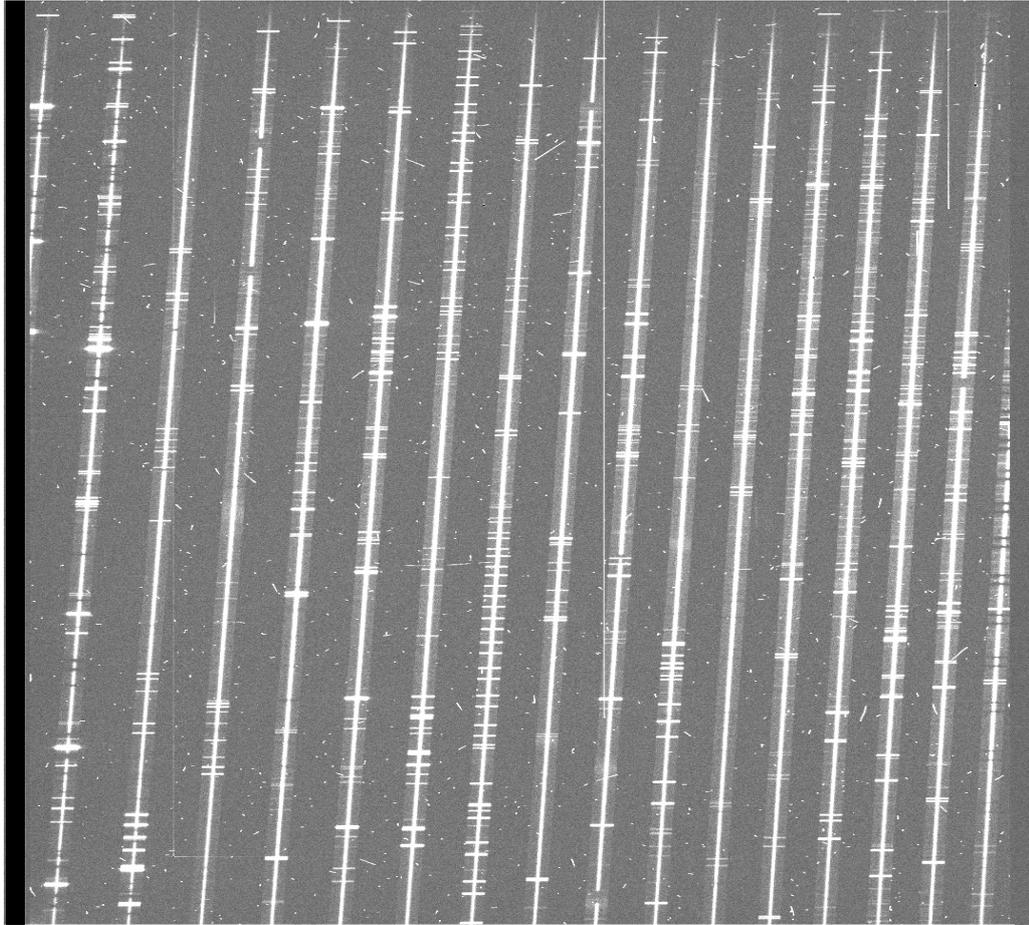
**Figure 1.6.** Example of a science frame collected with  $R \sim 40\,000$  echelle spectrograph. Each vertical line represents a different echelle order; each line shows part of a single quasar spectrum, which can be stitched together during the data reduction.
