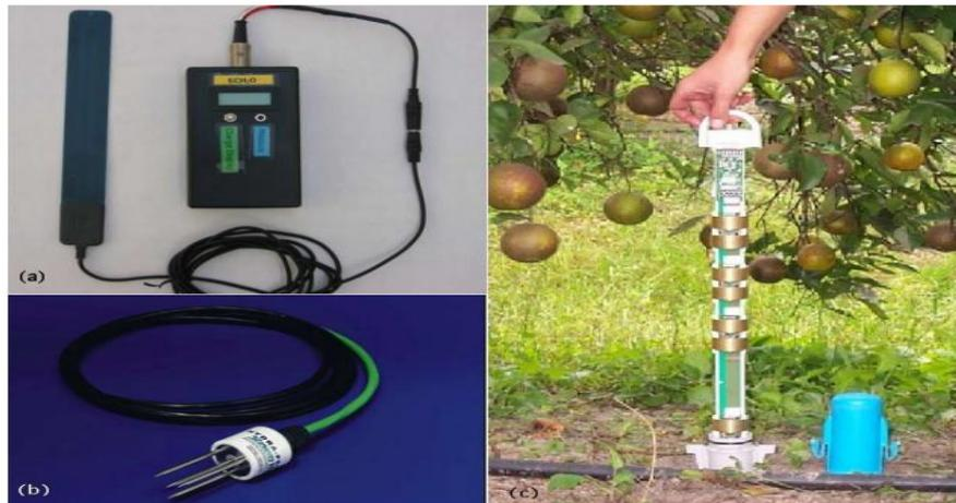
Figure 2.6. FD probes (a) Capacitance (plates) (b) Capacitance (rods) and (c) FDR (rings)
