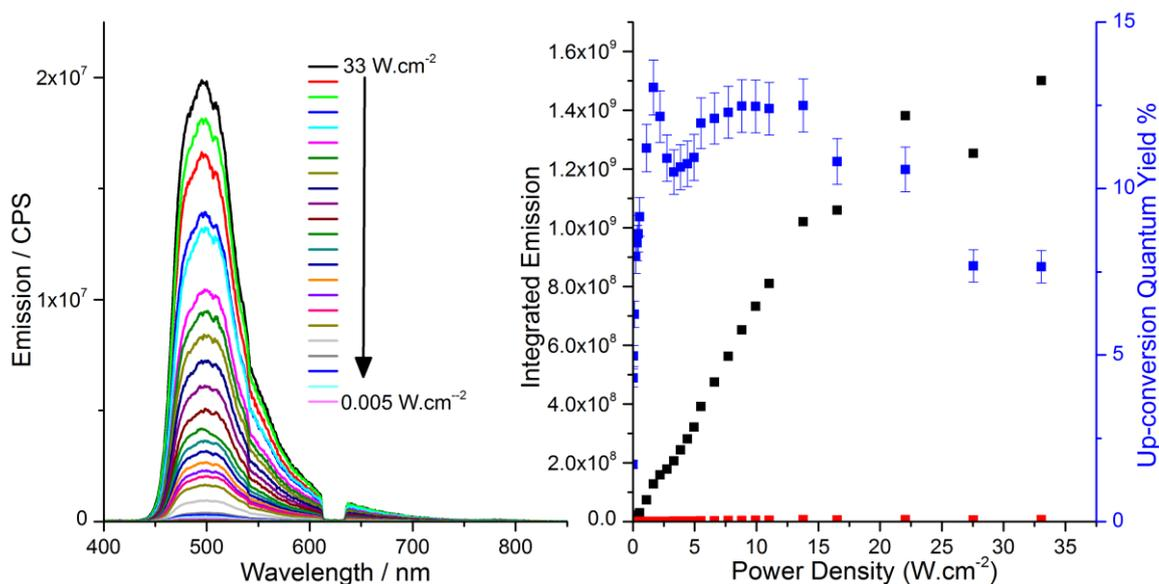
Figure 5.13 : Emission spectra (left) and integrated up-conversion (black) and sensitizer (red) emission, with up-conversion quantum yield (blue) of emitter **3h** ( $6 \times 10^{-4} \text{ M}$ ) and **PdTBP** ( $1.5 \times 10^{-5} \text{ M}$ ), excited by 633 nm varying intensity coherent photons
