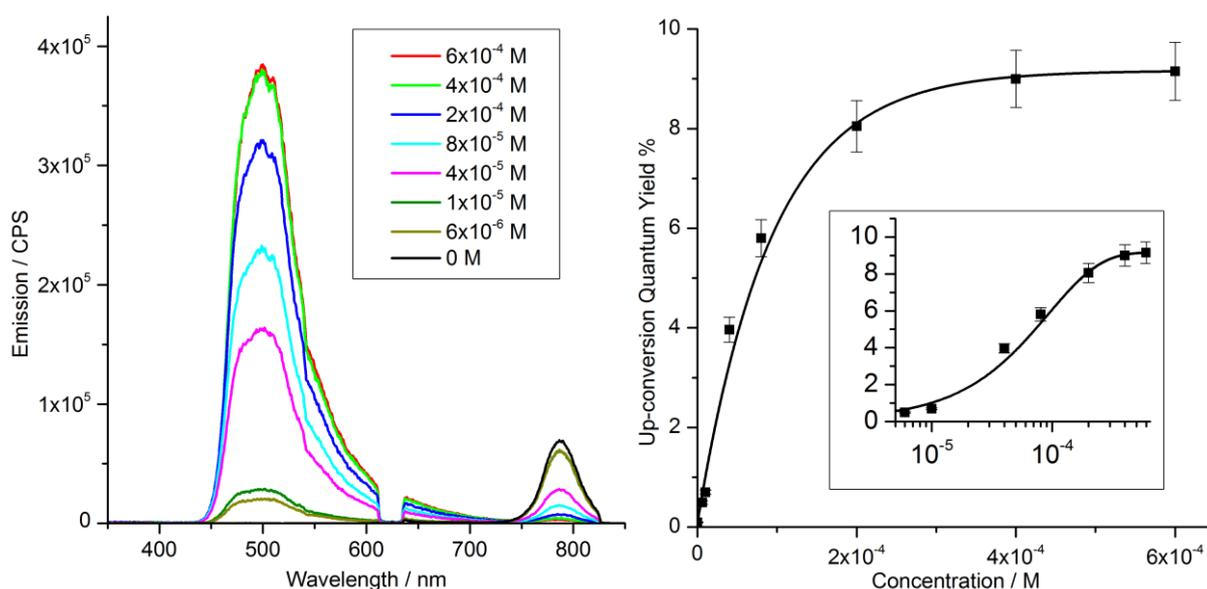
Figure 5.12 : Emission spectra (left) and up-conversion quantum yield of **3h** at varying concentrations, sensitized by **PdOEP** ( $1.5 \times 10^{-5}$  M) in dry, degassed toluene, excited by 532 nm 100  $\mu$ W ( $0.55 \text{ W.cm}^{-2}$ ) coherent photons
