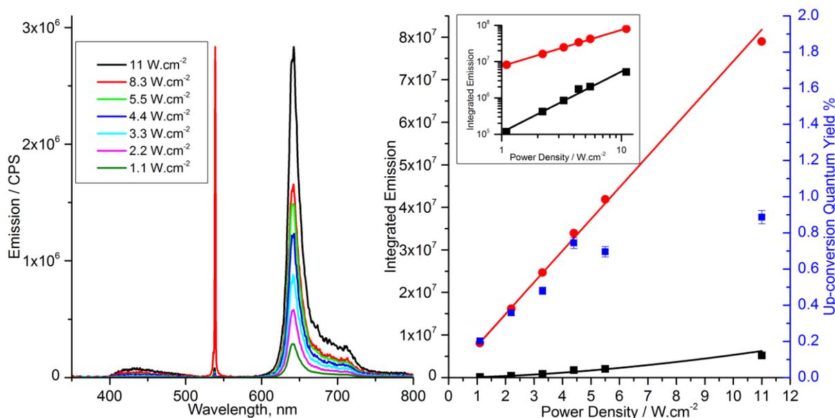
Figure 3.23 : Up-conversion emission spectra (left) and Integrated emission of up-conversion emission (black) and unquenched sensitizer emission (red) with double log plot inset (right) of **2h** ( $1.5 \times 10^{-5}$  M) and **PtOEP** ( $1.5 \times 10^{-5}$  M) in dry, degassed toluene, excited with varying intensity 532 nm coherent light
