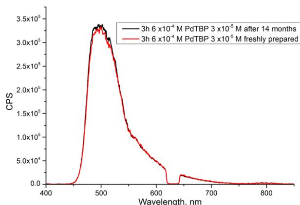
Figure 5.16 : Stability of up-conversion tube composed of **3h** and PdTBP
