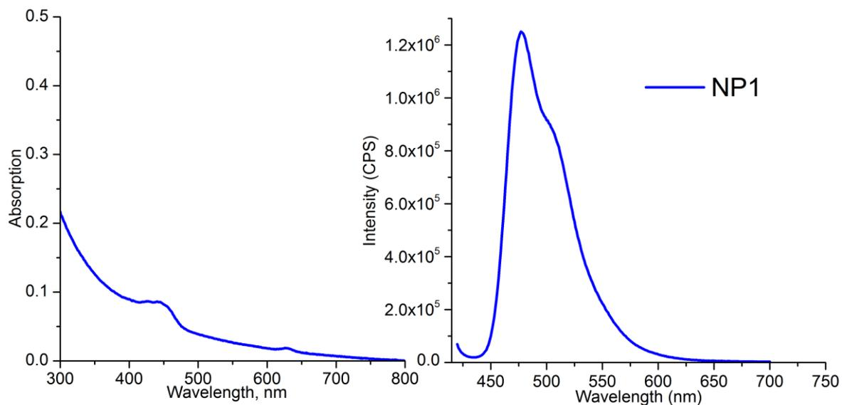
Figure 5.20 : Absorption (a) and emission (405 nm excitation) (b) spectra of nanoparticles dispersed in water
