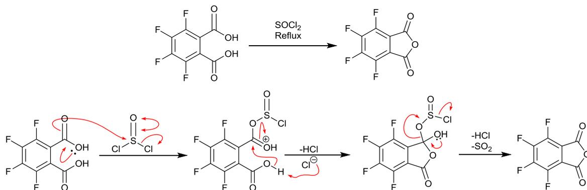
Figure 7.17 : Autodehydration reaction to form fluorinated intermediate tetrafluorophthalic anhydride
