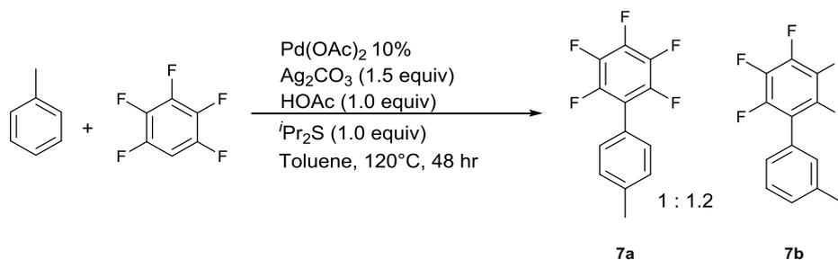
Figure 2.39: CH activated coupling of toluene with pentafluorobenzene
