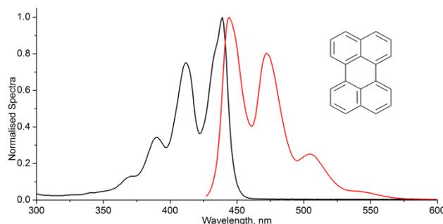
Figure 5.1 : Normalised absorption (black) and emission (red) spectra of perylene (toluene)
