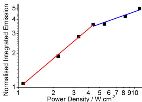
Figure 3.22 : Normalised integrated up-conversion emission against power density of **2h** and **PtOEP** (black) with linear fit lines of weak up-conversion limit (red) and strong up-conversion limit (blue).
