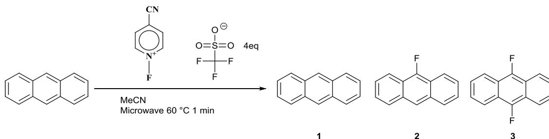
Figure 7.13 : Fluorination of anthracene by cyano-n-fluoropyridine
