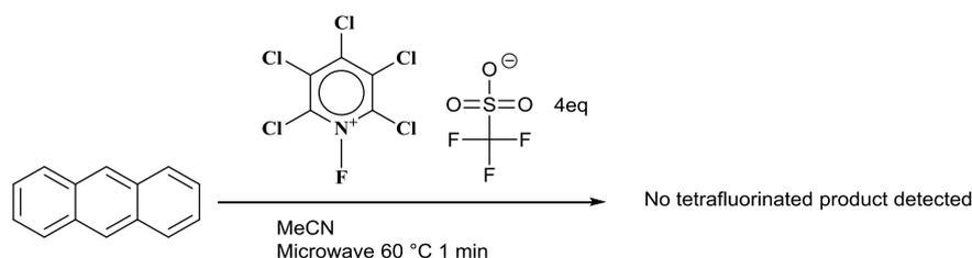
Figure 7.12 : Fluorination of anthracene by pentachloro-n-fluoropyridine
