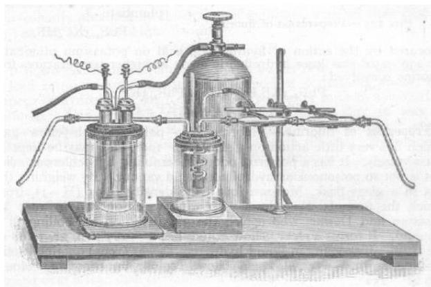
Figure 1.19 : Moissan's apparatus for the preparation of Fluorine, adapted from<sup>88</sup>
