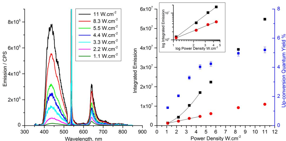
Figure 3.21 : Up-conversion emission spectra (left) and Integrated emission of up-conversion emission (black) and unquenched sensitizer emission (red) with double log plot inset (right) of **2h** ( $3.8 \times 10^{-4}$  M) and **PtOEP** ( $1.5 \times 10^{-5}$  M) in dry, degassed toluene, excited with varying intensity 532 nm coherent light
