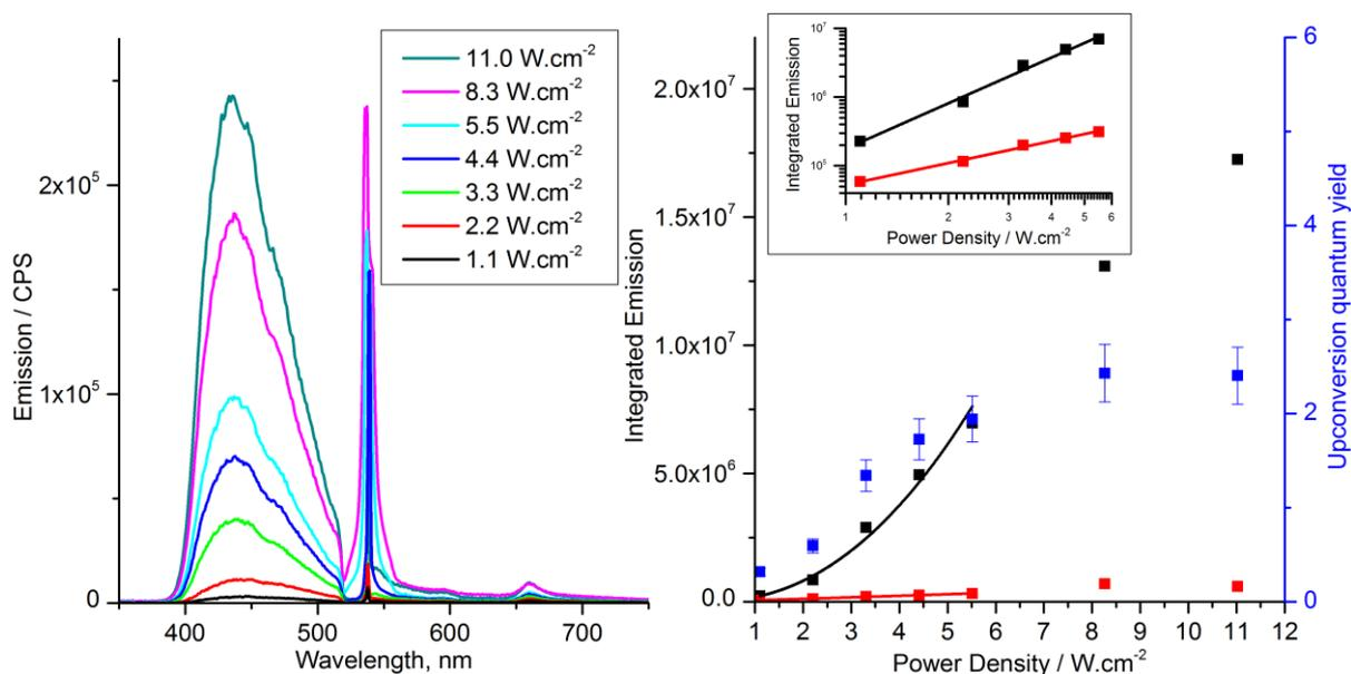
Figure 3.19 : Up-conversion emission spectra (left) and integrated emission of up-conversion emission (black) and unquenched sensitizer emission (red) with double log plot inset (right) of **2h** ( $3.8 \times 10^{-4}$  M) and **PdOEP** ( $1.5 \times 10^{-5}$  M) in dry, degassed toluene, excited with varying intensity 532 nm coherent light
