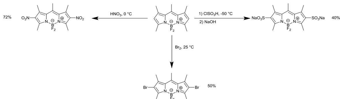
Figure 6.17 : Electrophilic substitution reactions on the BODIPY core, adapted from<sup>4</sup>
