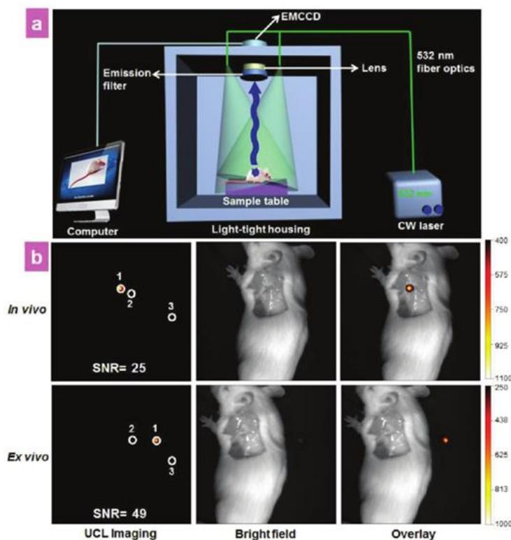
Figure 1.6 : a) Schematic layout of experimental setup. b) *In vivo* and *ex vivo* upconversion luminescence lymphatic imaging at 30 min postinjection of 20  $\mu$ l of TTAUC nanoparticles in paw (adapted from Li *et al.*<sup>60</sup>)
