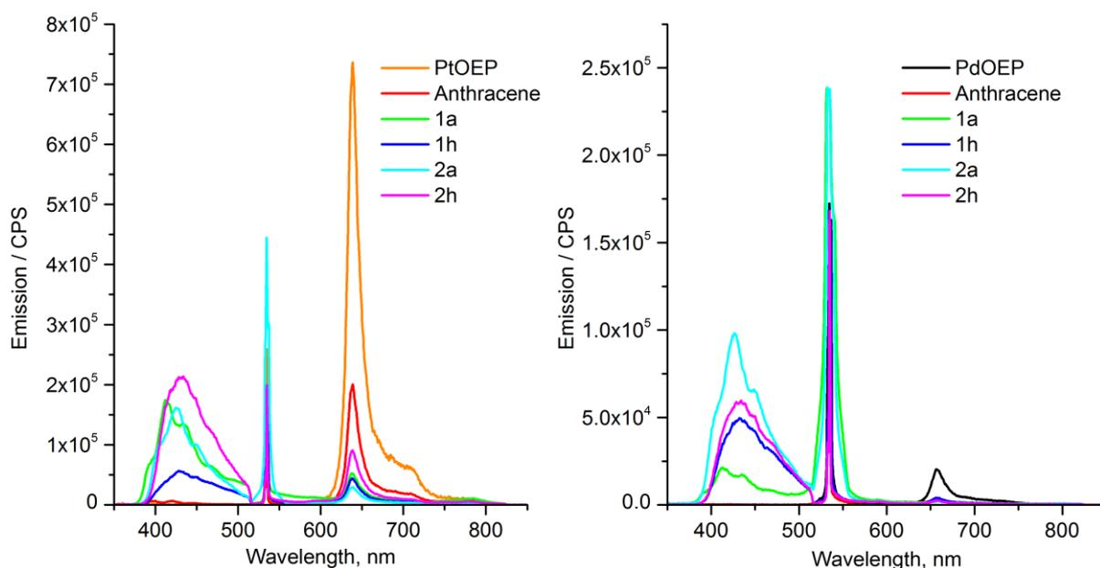
Figure 3.15 : Emission spectra of mixtures of each of emitters **A**, **1a**, **1h**, **2a** and **2h** with **PtOEP** (left) and **PdOEP** (right) excited with 532 nm 1 mW coherent light. The excitation region  $\sim 520 - 570$  nm is attenuated by a notch filter and is not integrated in quantum yield calculations.
