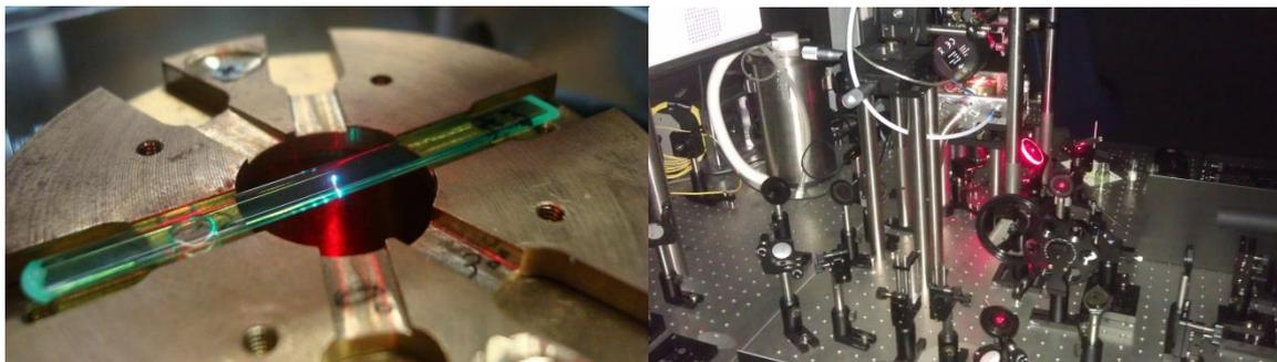
Figure 3.14 : Up-conversion tube in sample holder tilted at  $5^\circ$  (left) and sample holder apparatus and laser set up (right). Sample is **PdTBP** and **perylene**, illuminated with red light, emitting blue (see Chapter 5)
