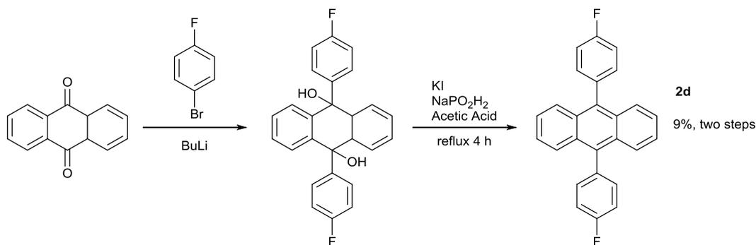
Figure 7.16 : Synthesis of diphenylanthracene emitter **2d** from anthraquinone
