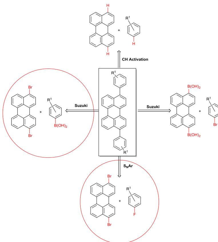
Figure 4.4 : Retrosynthetic analysis of bis-phenylperylene analogue synthesis
