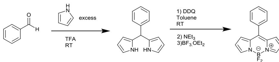
Figure 6.13 : Synthesis of simple BODIPY emitter
