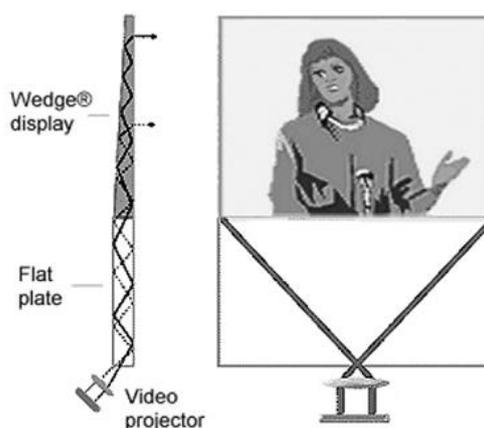
Figure 1.5 : Example side projection display (Cambridge Flat Projections Display Ltd.)<sup>62</sup>
