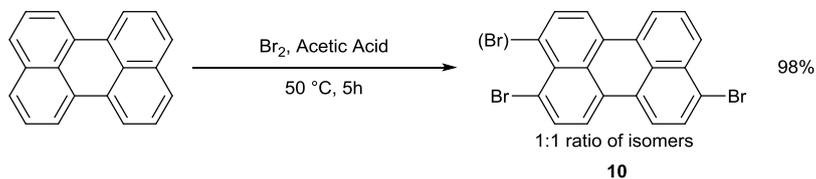
Figure 4.5 : Synthesis of dibromoperylene starting material
