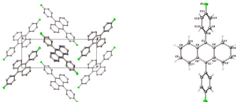
Figure 2.9 : Unit cell (left) and molecular structure (right) of **2d**, obtained by x-ray crystallography
