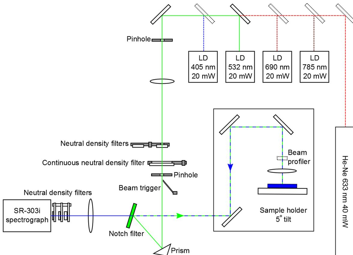
Figure 3.13 : Laser apparatus in Sony's Materials Science Laboratories for up-conversion measurements, with 532 nm laser diode in use. The beam paths of the other laser sources and mirrors not in use are shown by dashed lines.
