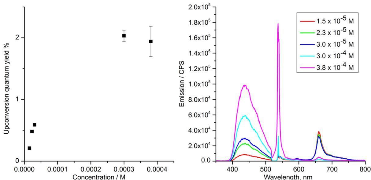
Figure 3.18 : Up-conversion quantum yields (left) and up-conversion emission spectra (right) of **2h** at varying concentrations with **PdOEP** ( $1.5 \times 10^{-5}$  M), excited with 532 nm 1 mW coherent photons,  $5.55 \text{ W/cm}^2$
