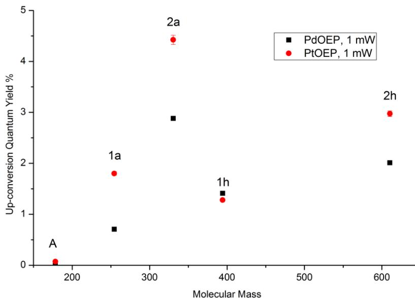
Figure 3.16 : Up-conversion quantum yields (%) of emitters **A**, **1a**, **1h**, **2a** and **2h** when sensitized by **PdOEP** (black) and **PtOEP** (red), excited with 532 nm 1 mW coherent light.
